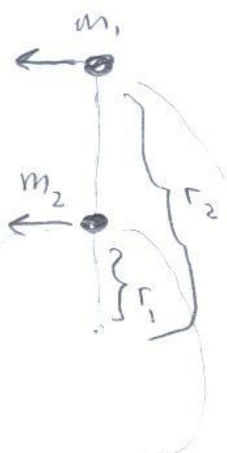
$$KE = \frac{1}{2} m_1 v_1^2 + \frac{1}{2} m_2 v_2^2$$
